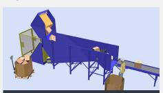
Without interrupting downstream processing, the buffering zone allows for continuous unloading of parcels while metering the flow for pre-singulation.
